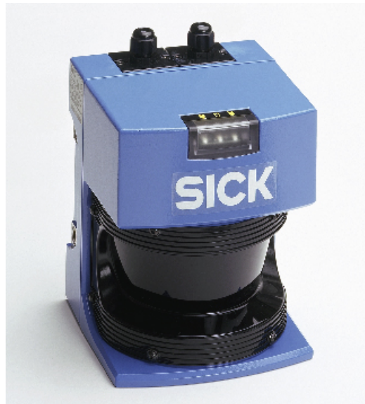
Figure 3.4: SICK LMS200 provides 361 distance measurements from 180 degrees angle range.
