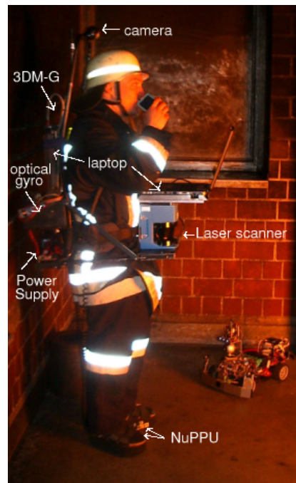
Figure 1.3: The PeNa system in operation. All the main components are pointed with arrows in the picture.
